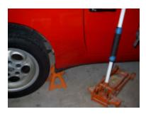
You will need a flat, safe area to perform the work. Be sure to use an adequate jack and reliable jack stands to support the rear of the 951. (Note the black pipe insulation on the jack handle to protect the car from dings.) Chock the front wheels. The jacks are placed on the outer ends of the swing arm pivot point.
